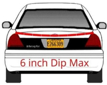
Ttrunk lid/tailgate may be welded, wired or banded in a 3 ON 3 Off Manner 3" x 3" x 1/8" plate maximum. The trunk may not overlap the quarter panels.
